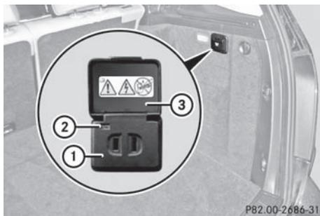
The 115 V AC power socket ① provides an alternating voltage of 115 V, so that small electronic devices can be connected. These
